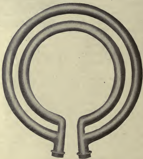
Fig. 20. Steam coils in Rogers pan Courtesy of C. E. Rogers
