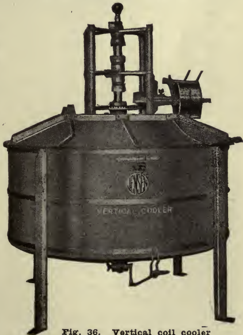
Fig. 36. Vertical coil cooler Courtesy of Jensen Creamery Machinery Co.
