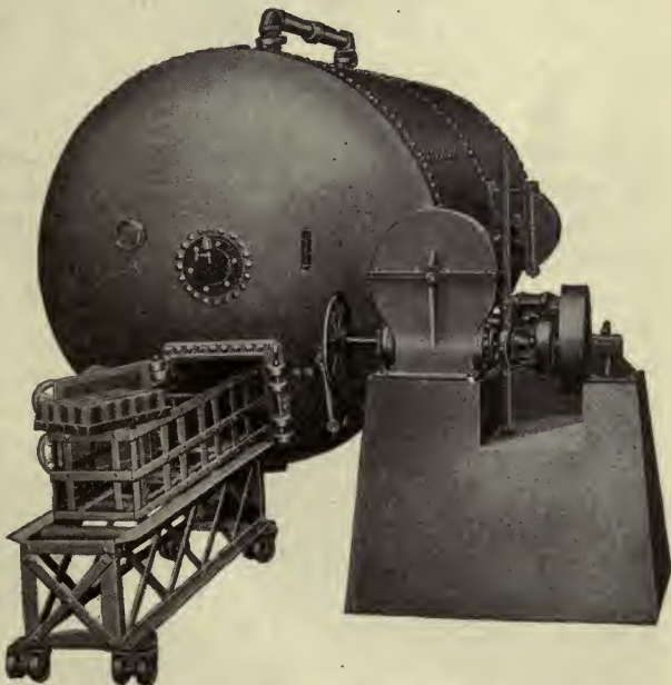
Fig. 59. Sterilizer for evaporated milk Courtesy of The Engineering Company
